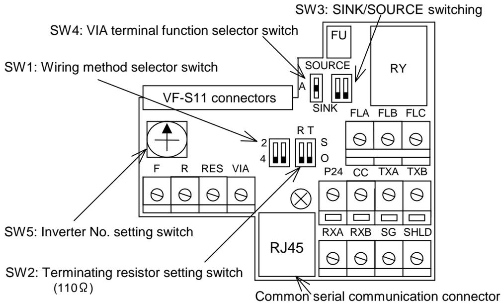
SW1: Wiring method (Set the two switches to the same side.)
