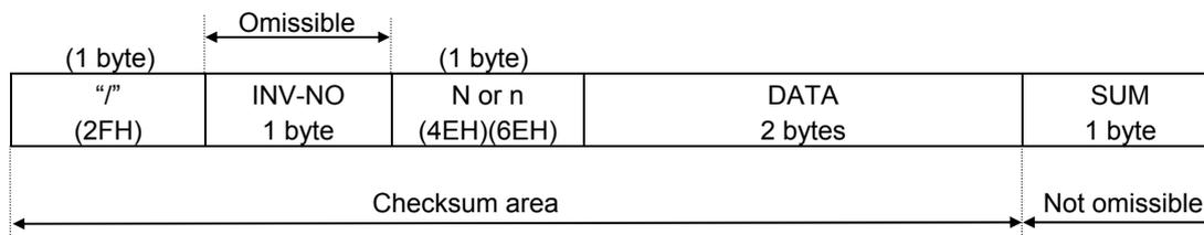
N or n (1 byte) : Communication error command ... This command is also used for a check when the inverter is tripped.
