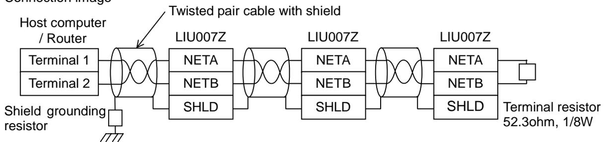
Network configuration is shown in the figures below. This LONWORKS communication option has TP/FT-10 channel type transceiver. The free topology wiring supported by the TP/FT-10 channel type accommodates bus, star, loop, or several combinations of these topologies shown in below
