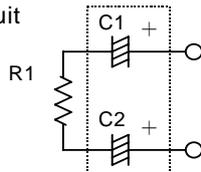
C1 and C2 are required for connection to link power network.
