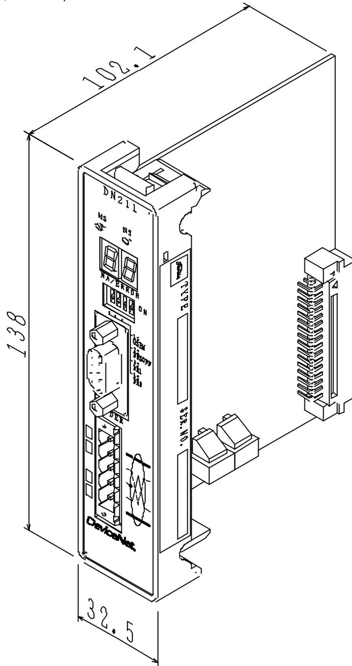
Figure 2.1 Outer Dimensions and Sizes (unit: mm)
