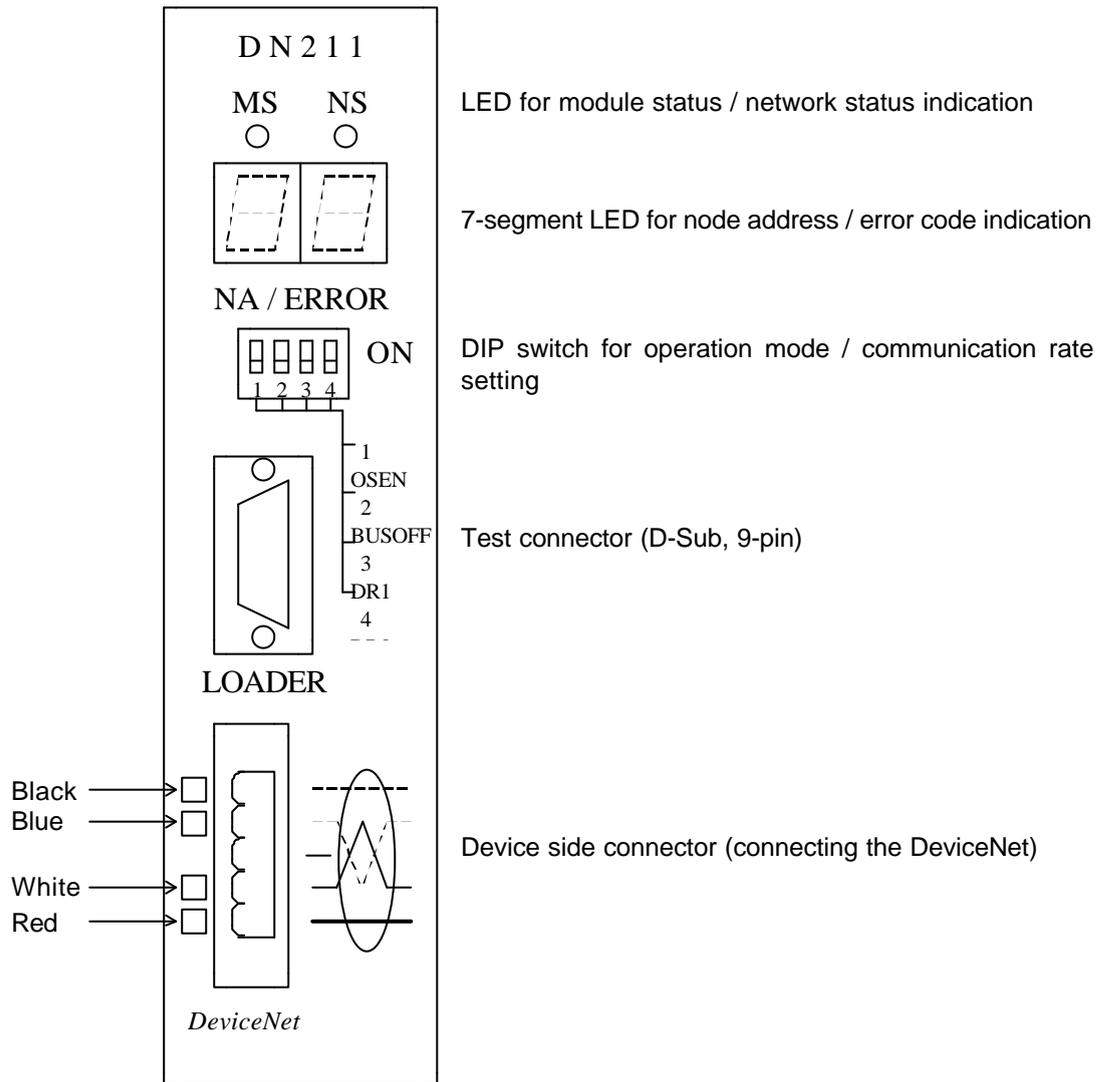
Figure 2.2 Appearance (front panel)
