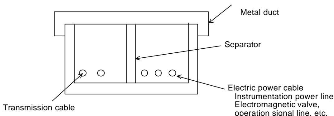
**Figure 8.1 Example of Installation in the Duct**
