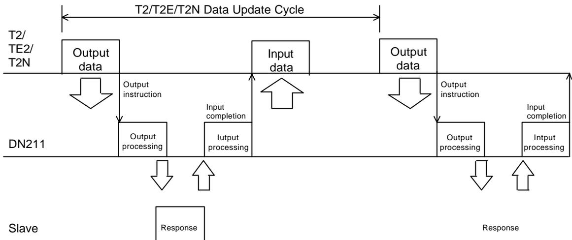
Output data and input data exchanged between the T2/T2E/T2N ↔ the DN211 are synchronizing with the output/input cycles of the T2/T2E/T2N side program. For this reason, the size of synchronous data value is equal to one-time output/input data to all slave devices.
