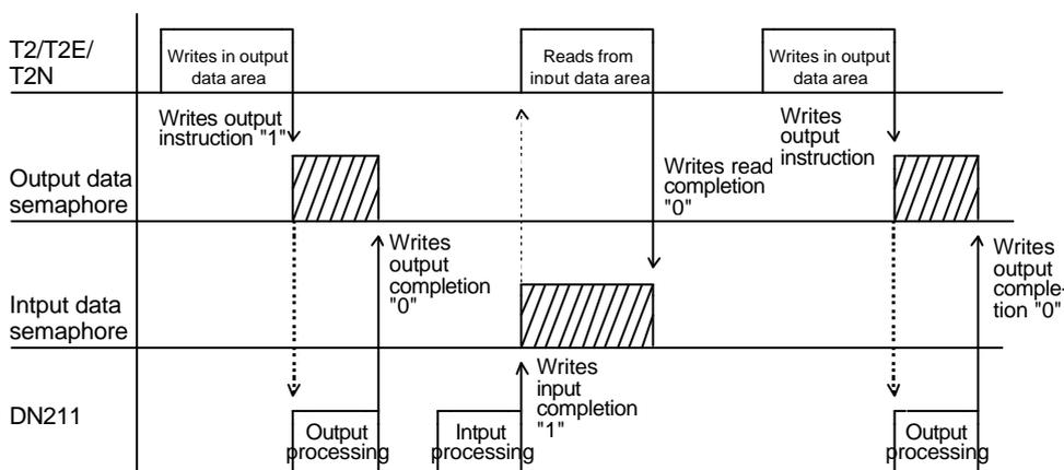
Figure 5.6 How to Use Semaphores in Synchronous Mode
