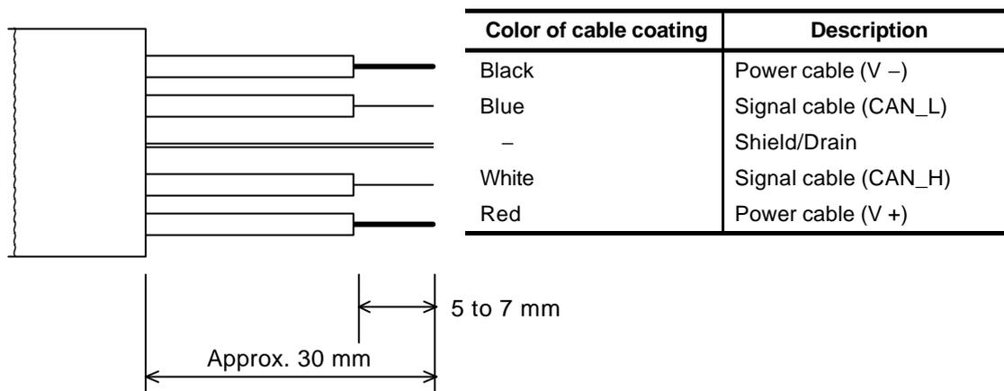
Figure 3.6 Processing of the DeviceNet Cable End
