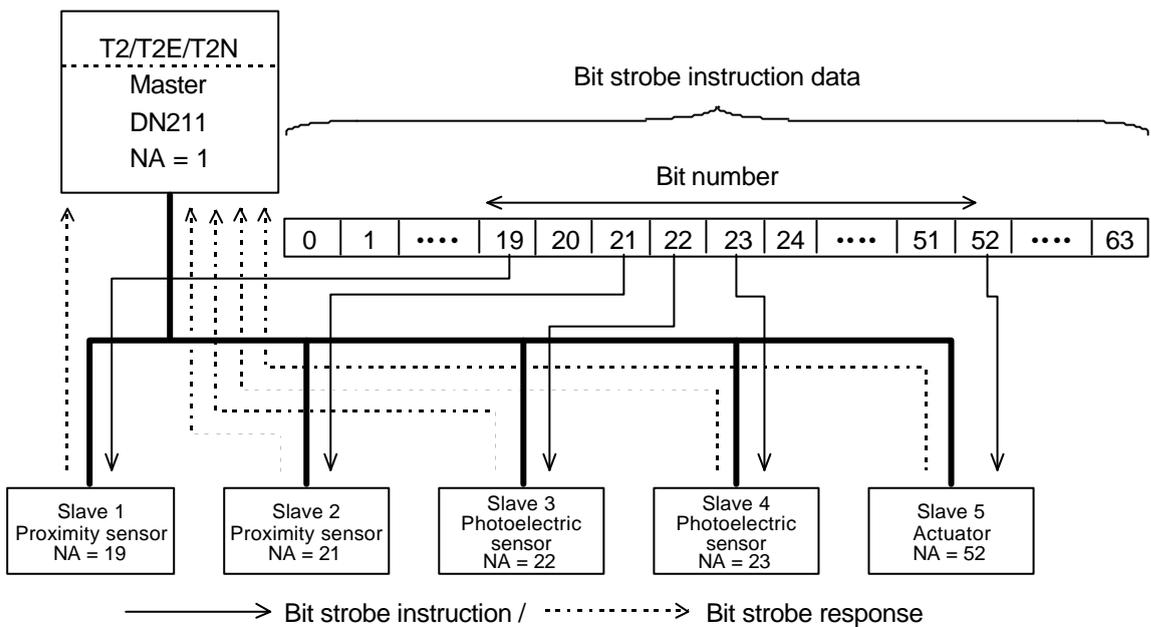
**Figure 1.9 Example of the Bit Strobe Instruction/Response Mode**
