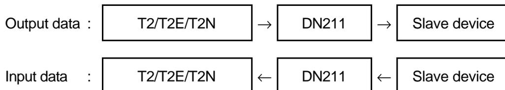
**Figure 1.1 Definition of Output Data and Input Data**
