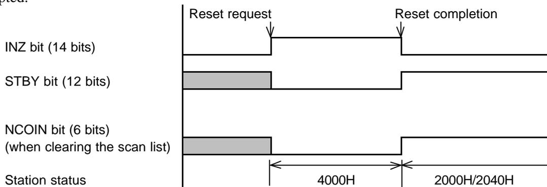
Figure 4.12 Station Status Operation on Reset Request
