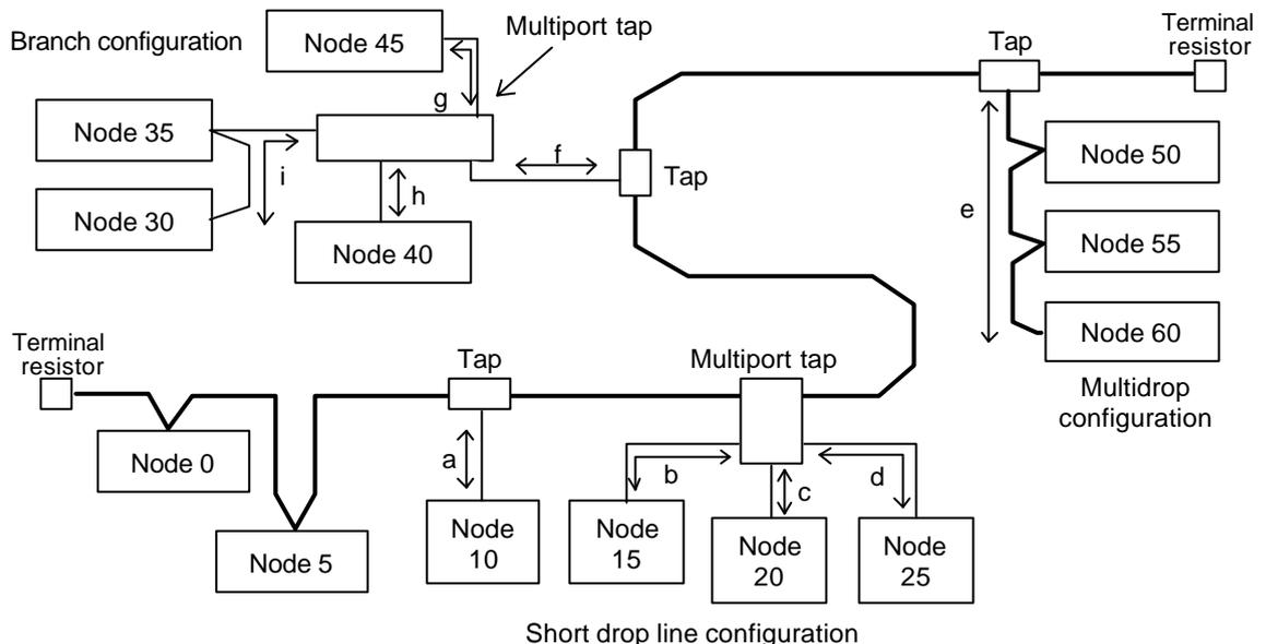
Individual drop line length:  $a \leq 6\text{ m}$ ,  $b \leq 6\text{ m}$ ,  $c \leq 6\text{ m}$ , and  $d \leq 6\text{ m}$  (short drop line configuration)
