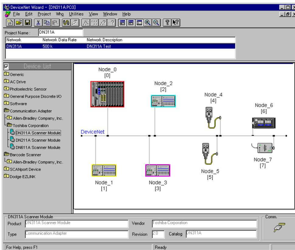
The personal computer in which DeviceNet Wizard for TOSHIBA is installed is connected with the DeviceNet network and actual, various work is done. There are three kinds of interfaces of the following by which the personal computer is connected with the DeviceNet network. Please buy the product from each maker's agency.
