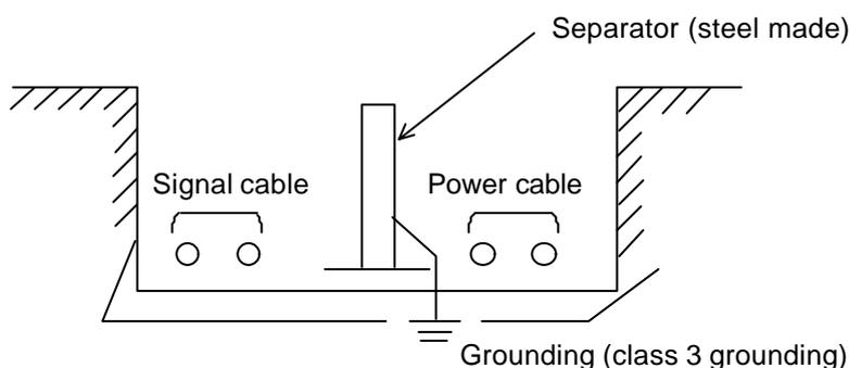
**Figure 8.2 Example of Installation in the Pit**
