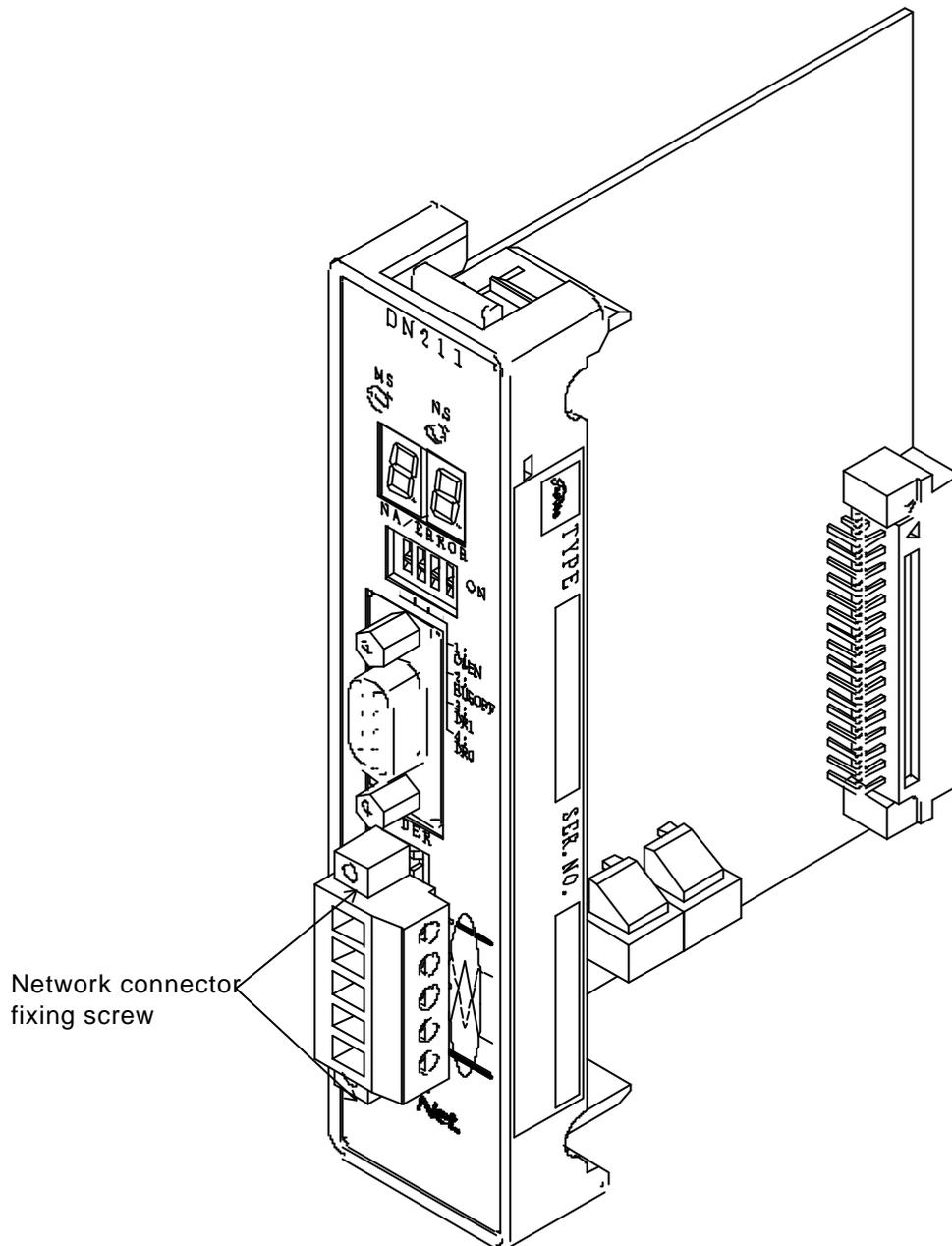
Figure 3.8 Mounting the Network Side Connector
