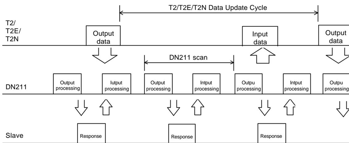
Transfer of output data and input data between the T2/T2E/T2N  $\Leftrightarrow$  the DN211 and the transfer between the DN211  $\Leftrightarrow$  slave devices are asynchronous. Transfer between the T2/T2E/T2N  $\Leftrightarrow$  the DN211 are synchronizes with the scan cycle by the T2/T2E/T2N side, while the transfer between the DN211  $\Leftrightarrow$  slave devices are synchronizes with the scan cycle in the DN211.
