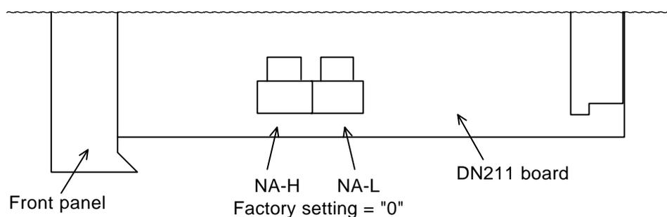
Figure 3.3 Rotary Switch for Node Address Setting
