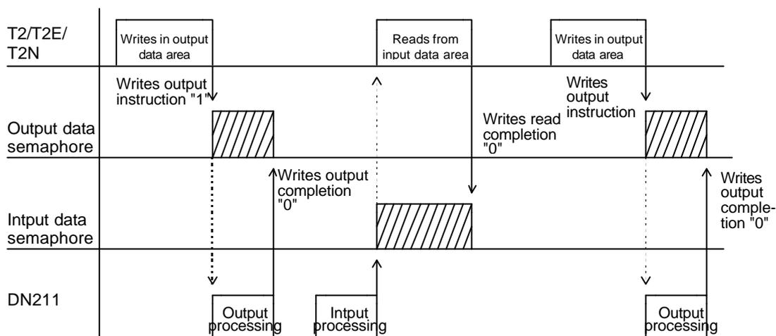
Figure 4.4 Use of Semaphores in Synchronous Mode
