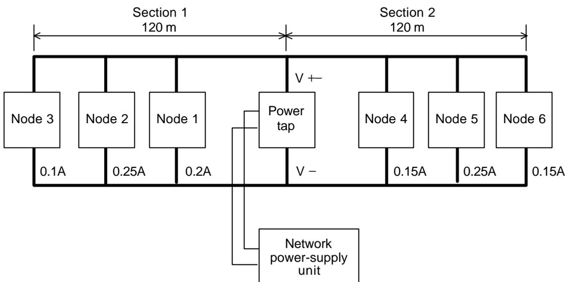
**Figure 3.13 Example of Single Power Unit Central Connection**
