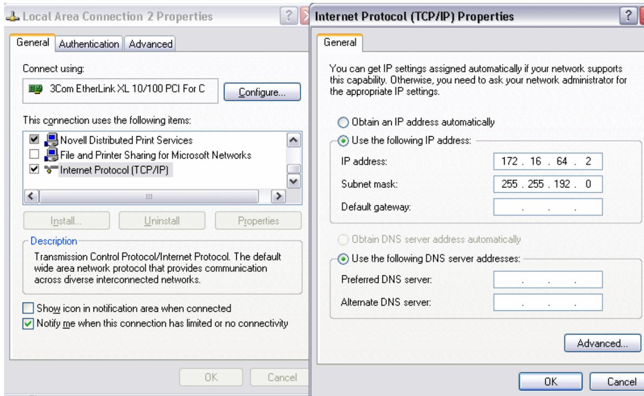
Note that the IP Address and Subnet Mast must be the same as set in T-PDS & the GEN651A (the last digit of the IP Address must be different however, it cannot be .1 The address of the GEN651A module is 172. 16.64.1 ). Click OK. In case of difficulty setting up the computer Ethernet card, contact the company MIS/IT Department.
