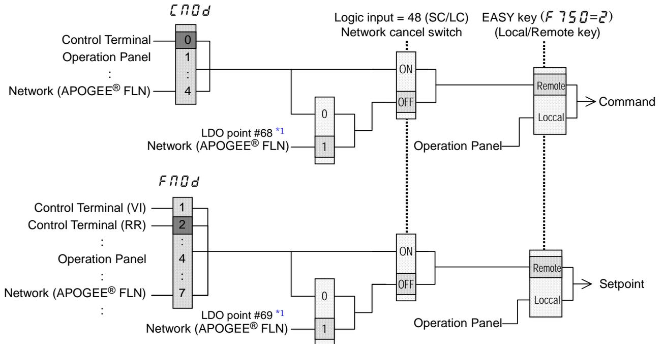
\*1 Be careful that *CNDd* command and *FNDd* setpoint are activated for a short time just after the inverter power turned on. Set *CNDd* and *FNDd* to “network” to prevent this problem.
