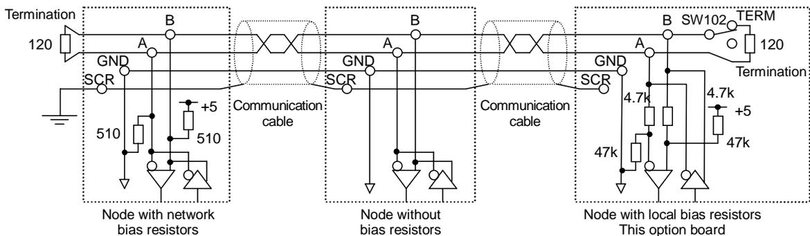
N.B.:Do not connect the SCR terminal to the power ground of inverters or other units.
