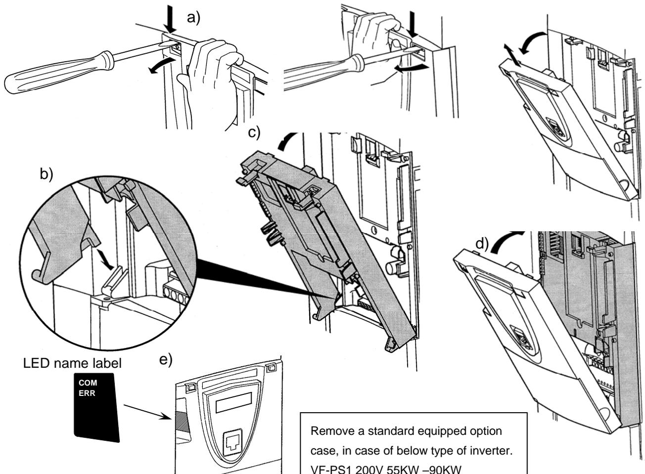
Remove a standard equipped option case, in case of below type of inverter.
