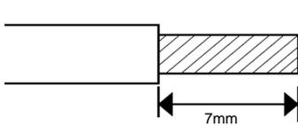
Cable sheath should be peeled off by about 7mm.
