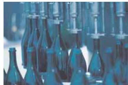
Automatic bottle shutting with torque limiting
