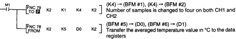
This step is the actual reading of the FX-4AD-TC input channels. It is essentially the only program step which is needed. The "TO" instruction in this example, sets the input channels, CH1 and CH2, to take the average reading of four samples. The "FROM" instruction reads the average temperatures (BFM #5 and #6) for input channels CH1 and CH2 of the FX-4AD-TC. If direct temperature readings are required BFM #9 and #10 should be read instead, e.g.
