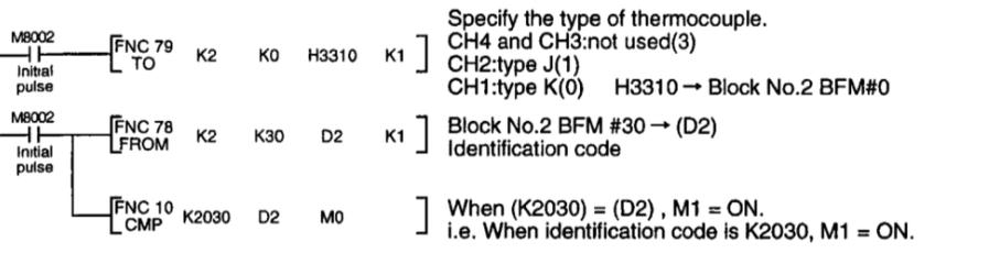
This initial step checks that the special function block placed at position 2 is actually an FX-4AD-TC, i.e. its unit identification number is 2030 (BFM #30). This step is optional, but it provides a software check that the system has been configured correctly.
